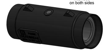
Richards 15/25 kV 600A Bushing Extender (P625BE) provides an insulated, fully shielded connection between an apparatus bushing and another 600A interface connection.
