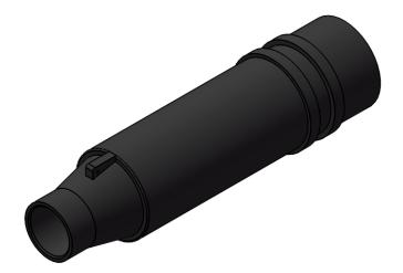
Richards Disconnectable Joints provide a robust, versatile option for splicing underground medium voltage cables. They can be used for straight or multi-way splicing and can be disconnected for circuit isolation, grounding, expansion and more. Disconnectable Joints are molded from peroxide-cured EPDM and are fully shielded and submersible.
