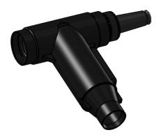
Richards 15 kV R800 (618MN) is a 600A elbow with a 200A loadbreak tap molded into the body. This combination design reduces the number of components, time, and effort required for installation.
