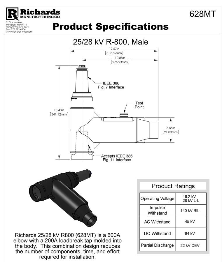
The R800 male version is fully shielded and features a male fastener for assembly to the bushing.
