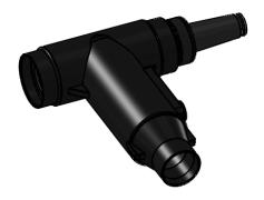
Richards 15 kV R800 (618MT) is a 600A elbow with a 200A loadbreak tap molded into the body. This combination design reduces the number of components, time, and effort required for installation.
