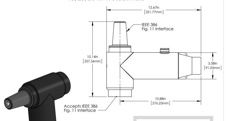
Richards 15/25/28 kV R-Stack (62CBT) is a 600A elbow with a 600A connecting plug molded in the body. This combination design reduces the amount of components, time, and effort required for installation.
