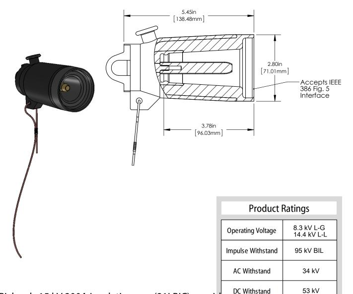
Richards 15 kV 200A Insulating cap (21LBIC) provides a means for shielding, sealing and insulating 200A loadbreak interfaces (IEEE 386, Fig. 5).
