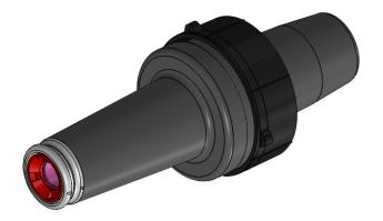
Richards 15 kV 200A Loadbreak Bushing Insert (21LBI) converts a 200A bushing well interface (IEEE 386, Fig. 3) to a 200A loadbreak interface (IEEE 386, Fig. 5) for use with a loadbreak elbow or cap.
